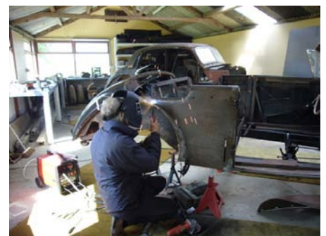
"Repairing rear wing roots"
